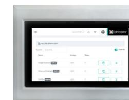
CD8 Pro controller supports unlimited recipe creation and editing, with the ability to name, version and track recipes over time. Optimised runs can be converted into reusable programs and a graphical preview helps users review steps before starting a run. Recipe usage tracking also supports process consistency and record keeping.
