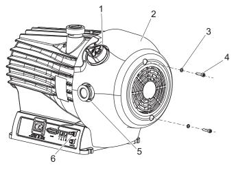
Fig. 25: Loosening the fan cover on the scroll pump
