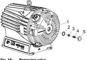
Fig. 19: **Removing valve**
