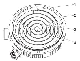
Fig. 29: Tip seal nut in the spiral housing
