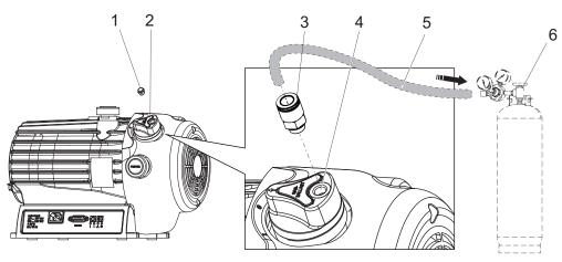
Fig. 8: Connecting gas ballast external supply
