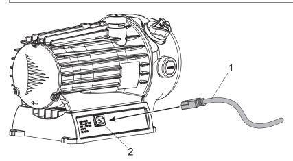
Fig. 9: Connecting to mains power supply
