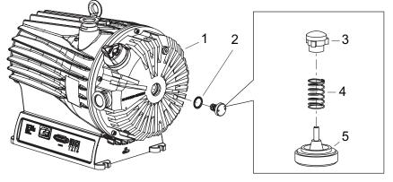
Fig. 20: Installing valve
