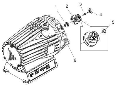
Fig. 21: Removing gas ballast valve
