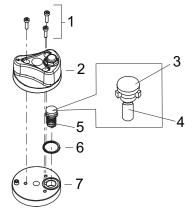
Fig. 23: Assemble gas ballast valve
