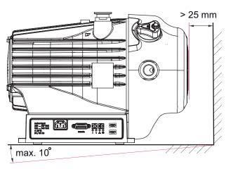
Fig. 5: Minimum clearances and permissible inclination
