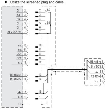
Fig. 11: Connection diagram of 15-pin "remote" connection
