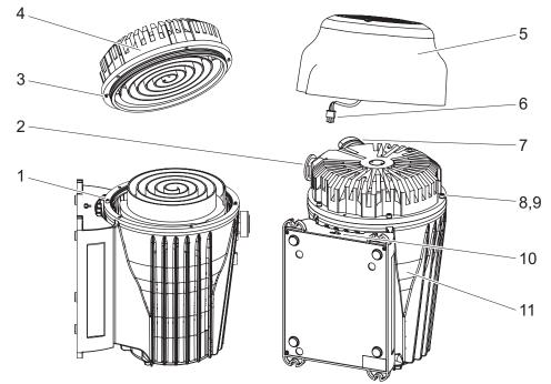
Fig. 30: Assembling the housing parts
