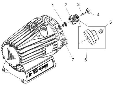
Fig. 24: Installing gas ballast valve
